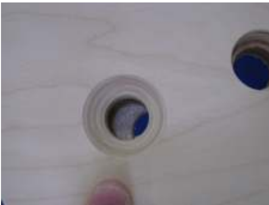
Sealing Processing Internal Borings Sealed
