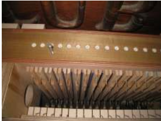
Main Slider Chest: Note Construction Matches Unit Chests
