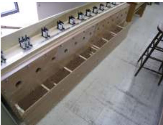
Unit Wind Chest With Magnets Attached
