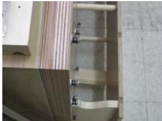
Unit Wind Chest: Note Wood Laminate
