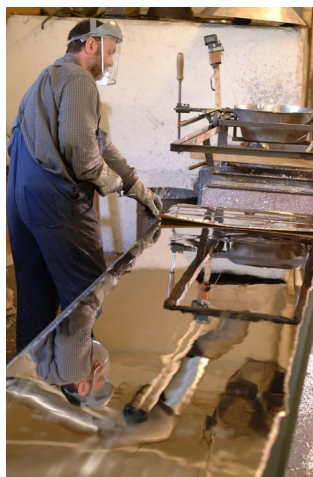
When the metal cools it can be carefully peeled up.
