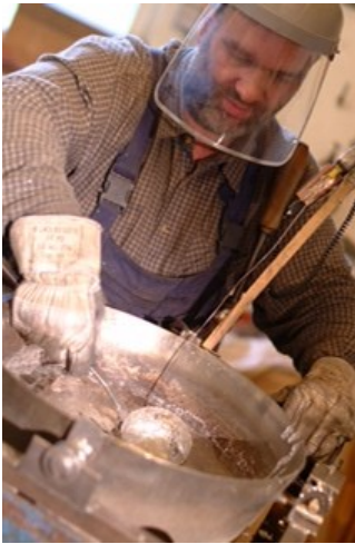
Metal shards (typically a combination of tin and lead) are melted in a vat.
