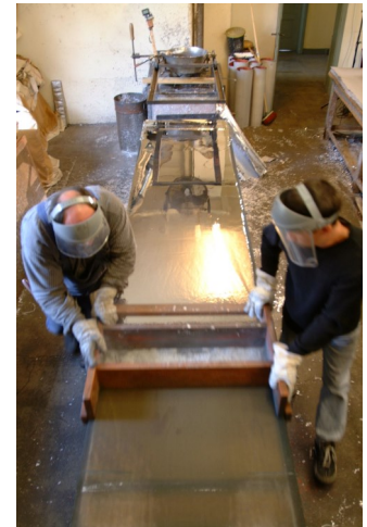
Two craftsmen slide the box along a counter as the molten metal runs out the slit creating a thin layer of metal.
