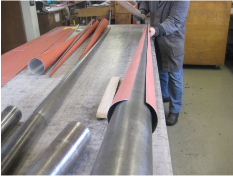
Using a mandrel, the sheets are formed into pipe shapes. Here the bottom half of an organ pipe is being formed.
