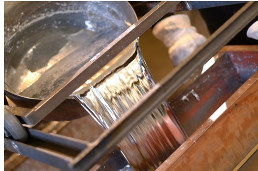
The molten metal is poured into a wooden box with a thin slit at the bottom.
