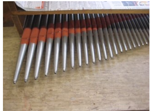
Here are pipes that have been soldered together. The bottoms of these pipes (the "toes") are made to make their characteristic shape—a tapered toe that will sit in its hole in the pipe rack.
