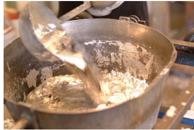
Metal shards (typically a combination of tin and lead) are melted in a vat.
