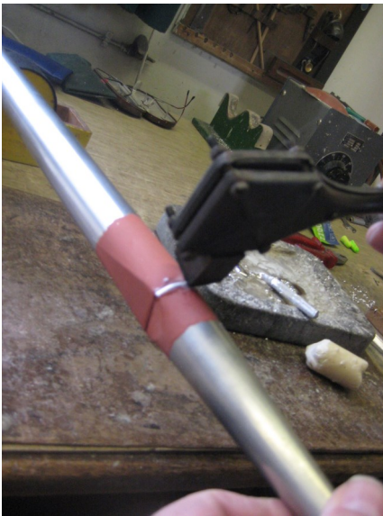
Each pipe is hand soldered. The pipe is painted with more sizing, and the sizing is scraped off in the exact area where the solder is to be applied. This way the solder does not run all over the pipe.
