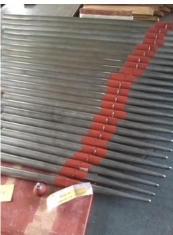
These pipes have been soldered but will still need the "mouths" (the side openings) cut into them.
