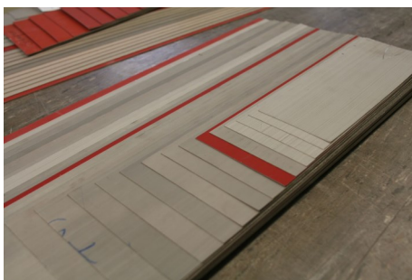
The sheets are painted with a gum-like sizing on one side and after seasoning for three months are ready to be molded into pipes.
