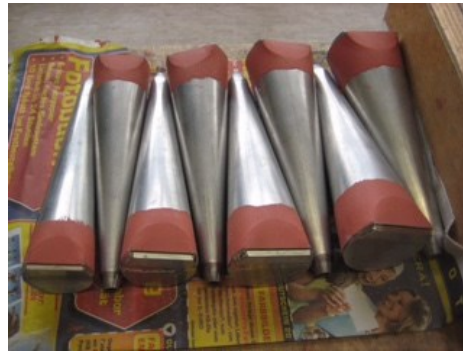
These pipe bottoms are ready to be soldered to their tops. The indented part of the pipe (which is the bottom half of the pipe's mouth) has been formed by hand.
