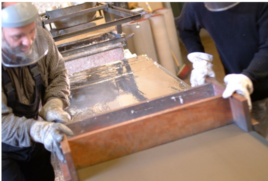
When the metal cools it can be carefully peeled up.
